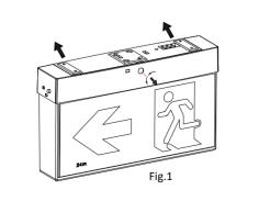
Use a tool to take off the Round locking tab from the base; Remove the plate by sliding it away;
