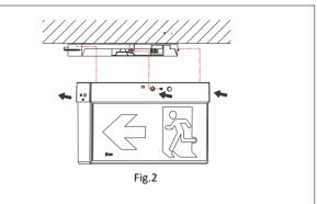
Asemble the body to the base, then push the round locking tabs back in with supplied screw, to complete the process.
